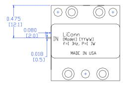
Unit: INCH Base Material: Brass [mm] Finish: Gold Plating Tolerance: X.XX ±0.01" X.XXX ±0.005"
